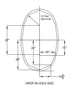
Note: The pump extends approximately 1" past the end radius of the bath. This requires angling the bath into the drop-in hole.
