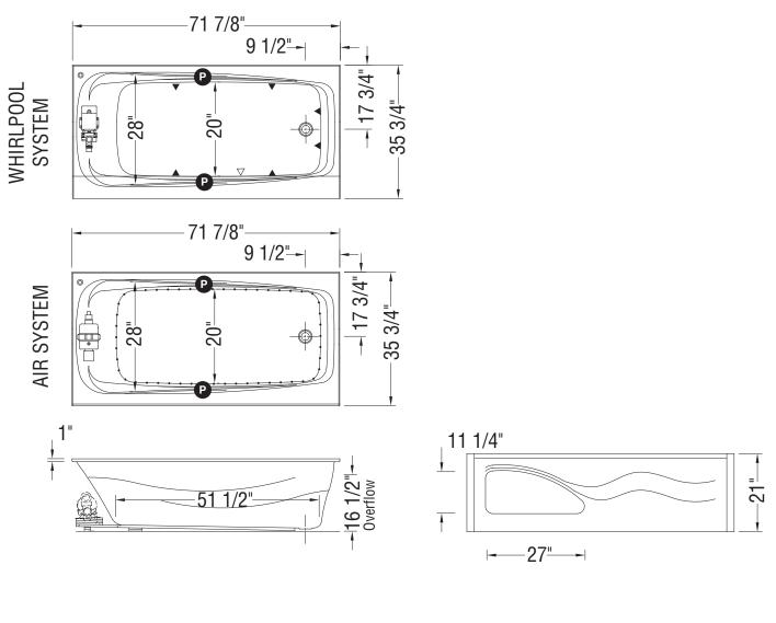
△ ): Indicates suction positioning All dimensions are approximate. Structure measurements must be verified against the unit to ensure proper fit.
