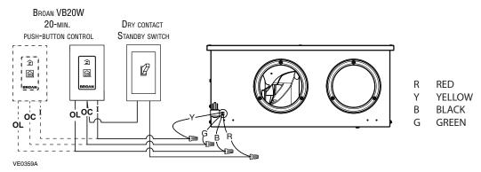
This connection allows the operation of VB20W push-button controls even if the dry contact standby switch is turned off.
