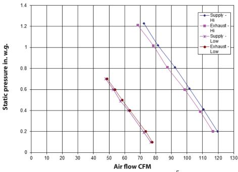
Note: In high speed, account for an increase in static pressure of proximately 0.2 in. w.g. when installed with the Broan VTYIK1 Tandem transition, depending on installation.
