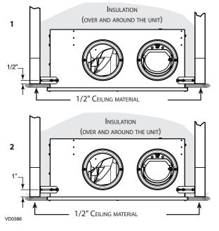
Refer to Installation and User guide for more details on installation in zone B with a surrounding sealed enclosure.
