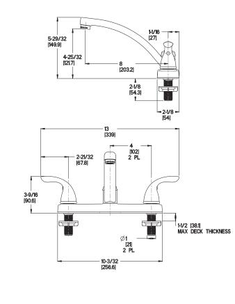
Ø1-3/8 Min to Ø1-1/2 Max. Deck Hole Openings
