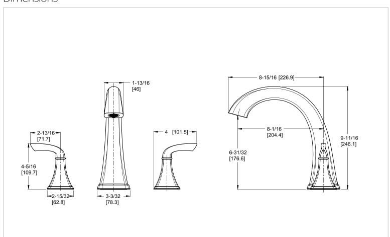
Ø1 Min to Ø1-1/2 Max. Deck Hole Openings
