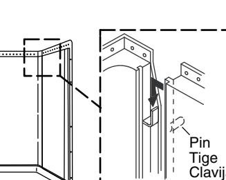
**15 The front edges should be flush, with no more than a 1/32" (1 mm) gap.**
