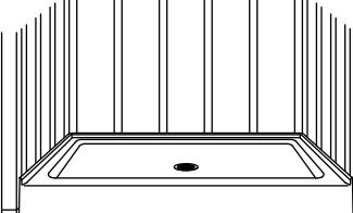
**11 STERLING Wall Set: Install the back wall. Insert the tabs into the slots.**
