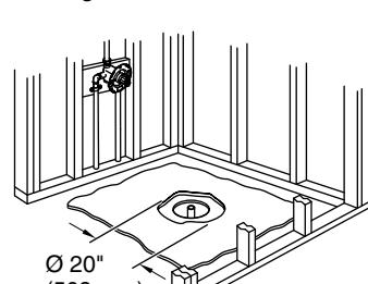
**7 With the unit level, shim under the support feet as needed.**
