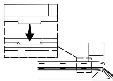
Install on an adequately supported subfloor.
