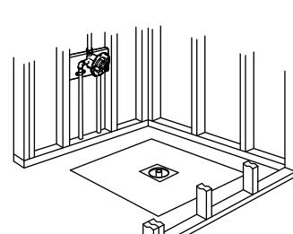
With no pad, lay a 1/4" (6 mm) mortar cement bed with a 20" (508 mm) diameter space around the drain.
