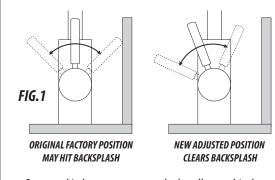
Unscrew and remove metal cap (A) and Hot and Cold Indicator Ring (B). Unscrew and remove holding screw (C) and washer (D). Hold handle (E) in a vertical position. Wiggle and pull straight off faucet. Rotate handle 22 degrees away from backsplash then slide handle back onto valve stem (F). Insert holding screw with washer and tighten. Slide Hot and Cold Indicator Ring onto handle and thread metal cap back into place. To adjust handle tension, turn ring (G) clockwise to increase
